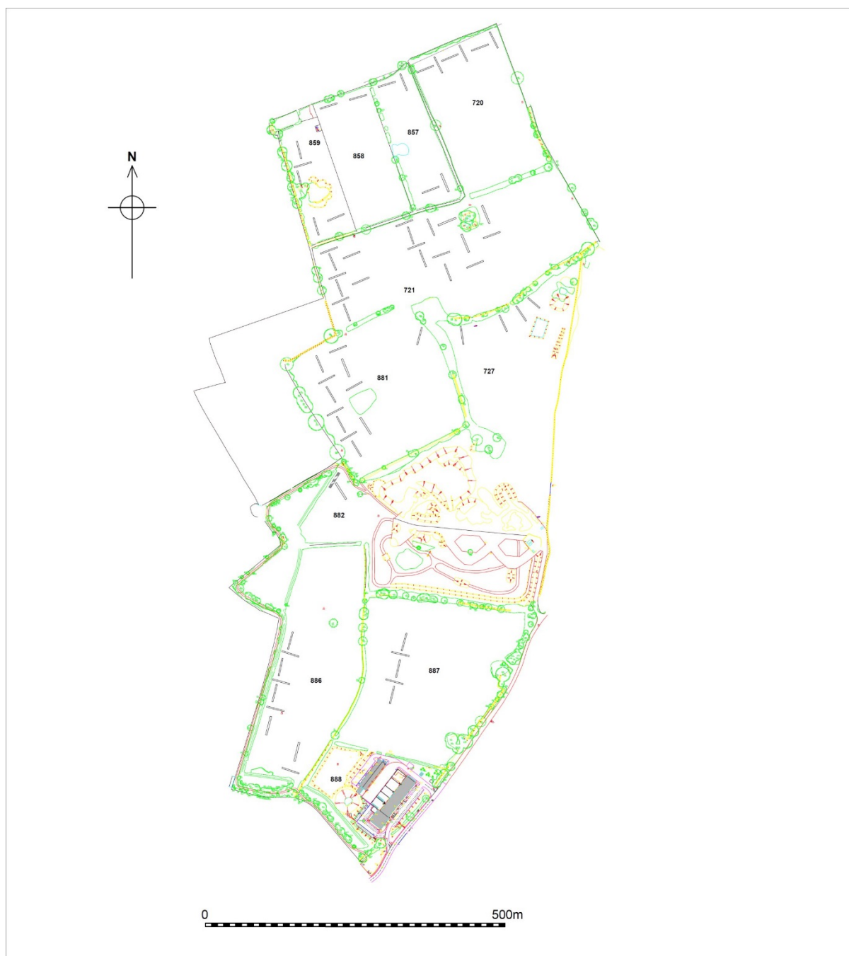
Figure 3: Final trench layout across the proposed TIC-IT site with field numbers
