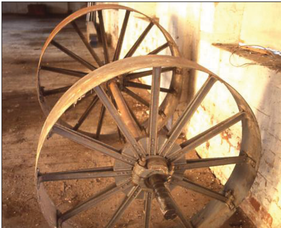
Plate 14 Part of lift power mechanism originally on top floor
