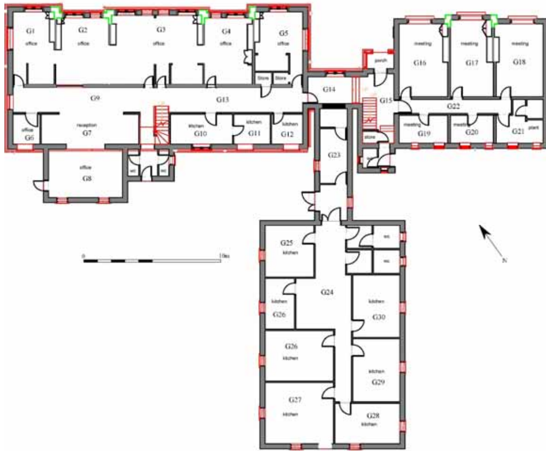
Figure 30 Freeman's Cottages ground floor plan Modified from plan supplied by client. Room identification letters used for this survey only and do not relate to earlier uses
