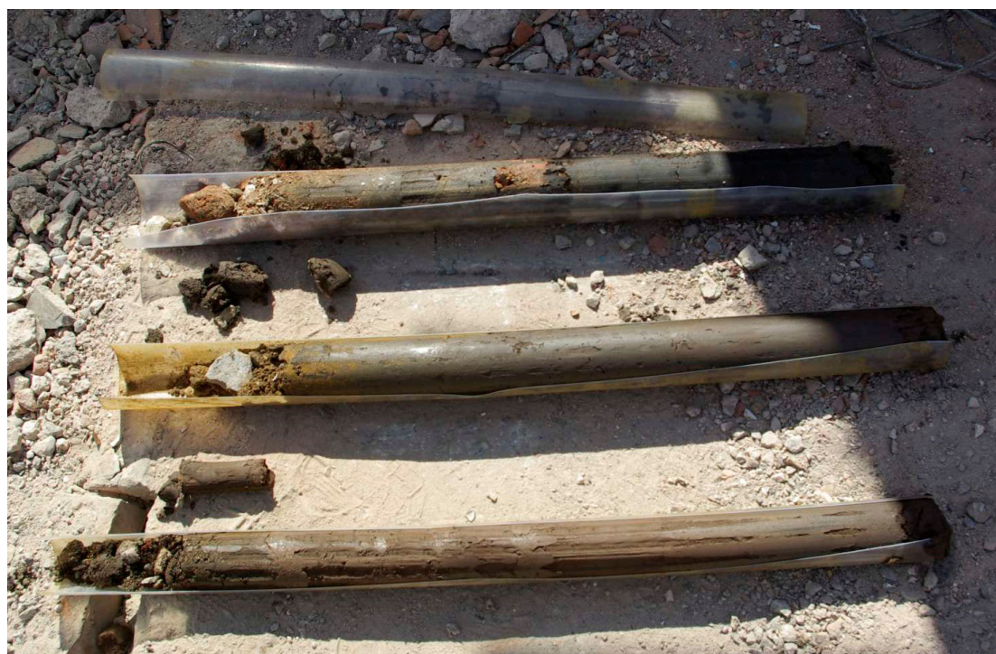
Figure 4 Core samples from Borehole 101 1 metre long tubes. Highest level at top left, deepest sample bottom right
