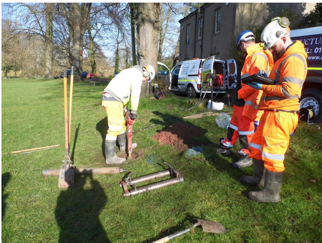
Figure 8: Excavation of Window Sample 1.
