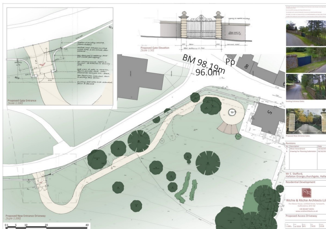
Figure 3: Plan of proposed access driveway, passing places, turning circle and parking bay. Plan provided by client.
