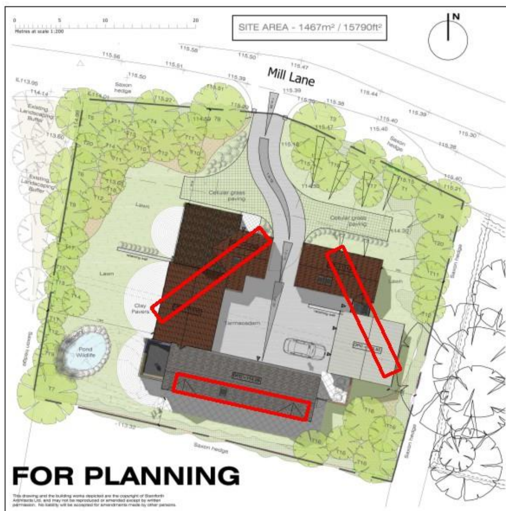
Figure 4: Trench plan overlaying the proposed construction.
