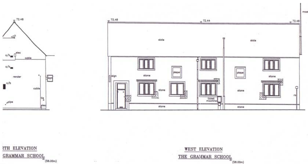
Fig. 4: Proposed areas for removal of concrete render to door and window surrounds, 6 areas in total
