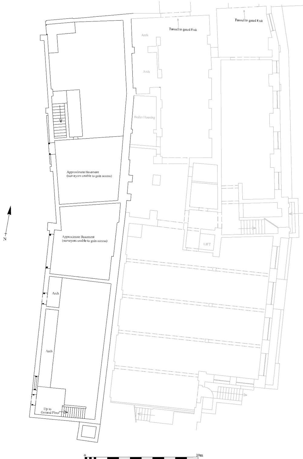
Figure 28 Plan of 10 Short Hill basement Adjacent buildings not part of demolition shown in grey Modified from client's drawings
