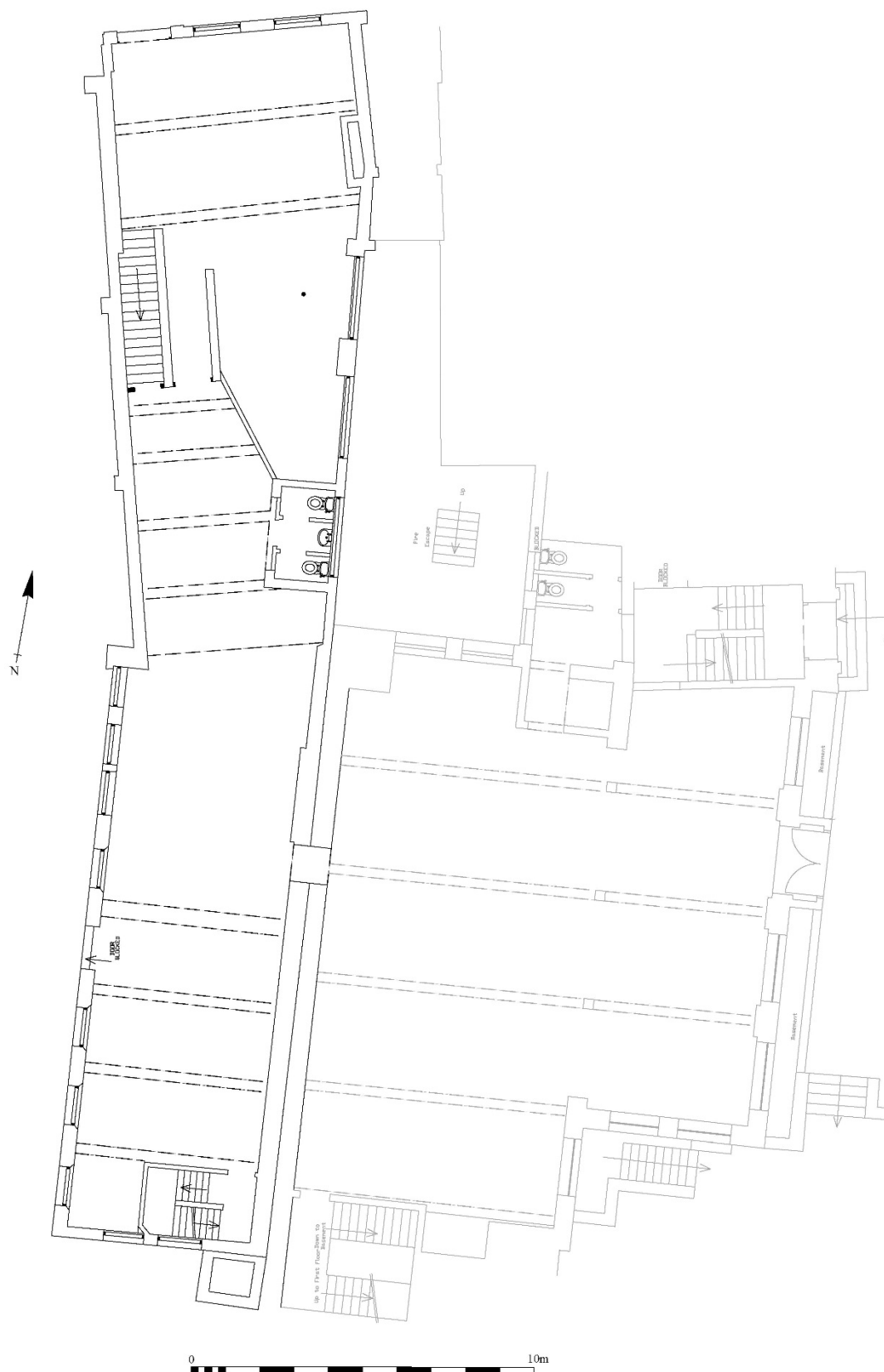
Figure 29 Plan of 10 Short Hill ground floor Adjacent buildings not part of demolition shown in grey Modified from client's drawings
