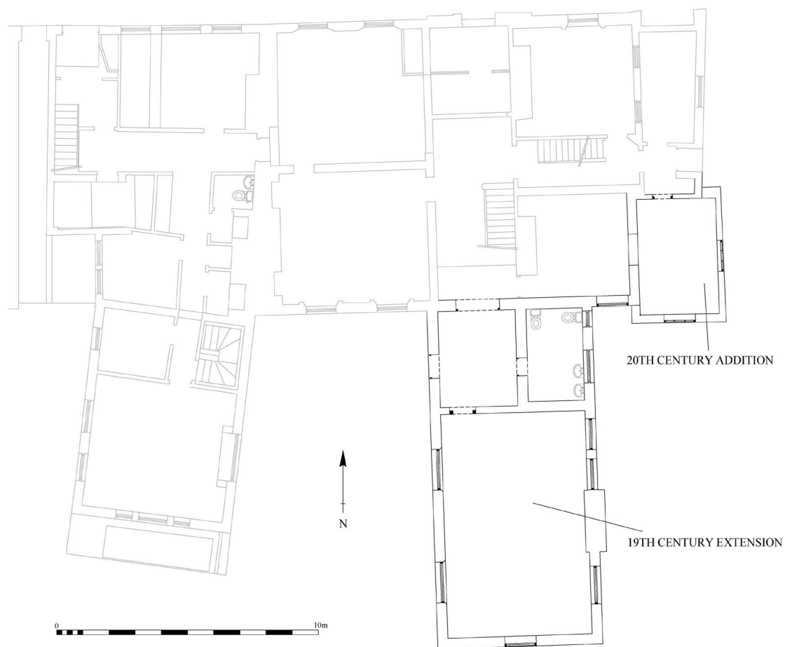
Figure 46 Overall plan of 54-56 High Pavement Adjacent buildings not part of demolition shown in grey Modified from client's drawings
