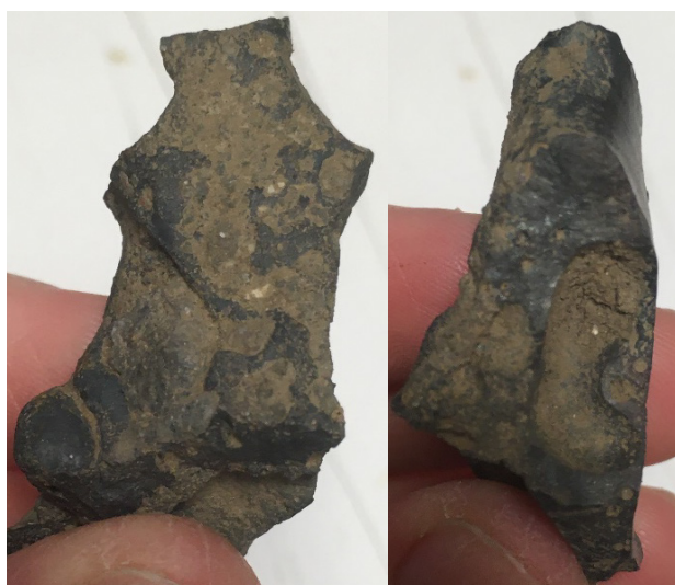
Figure 24: Iron tap (smelting) slag from (13) showing flowing appearance on top (left) and density in section (right).
