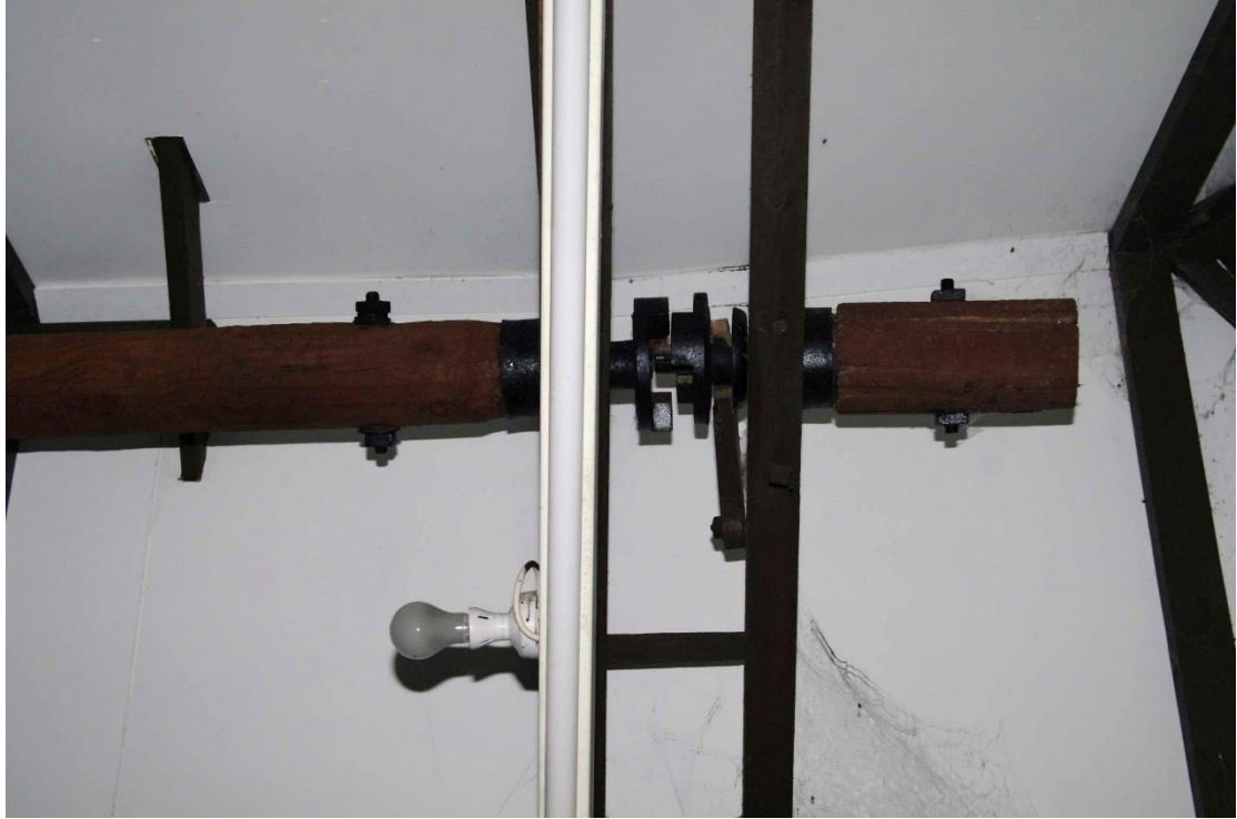
Figure 107: Dog clutch on the sack hoist Northern end of the mechanism
