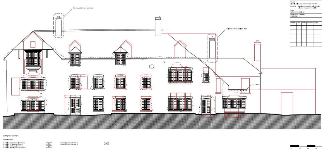
Figure 47: WGP overlay of earlier features over current south-east facing elevation Earlier features shown in red. Source WGP 2020
