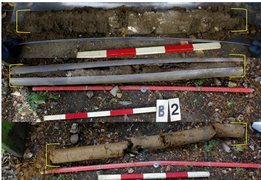
Figure 7 B2 borehole samples Samples highlighted by yellow brackets. 0.5m scale. Upper ends of samples to left
