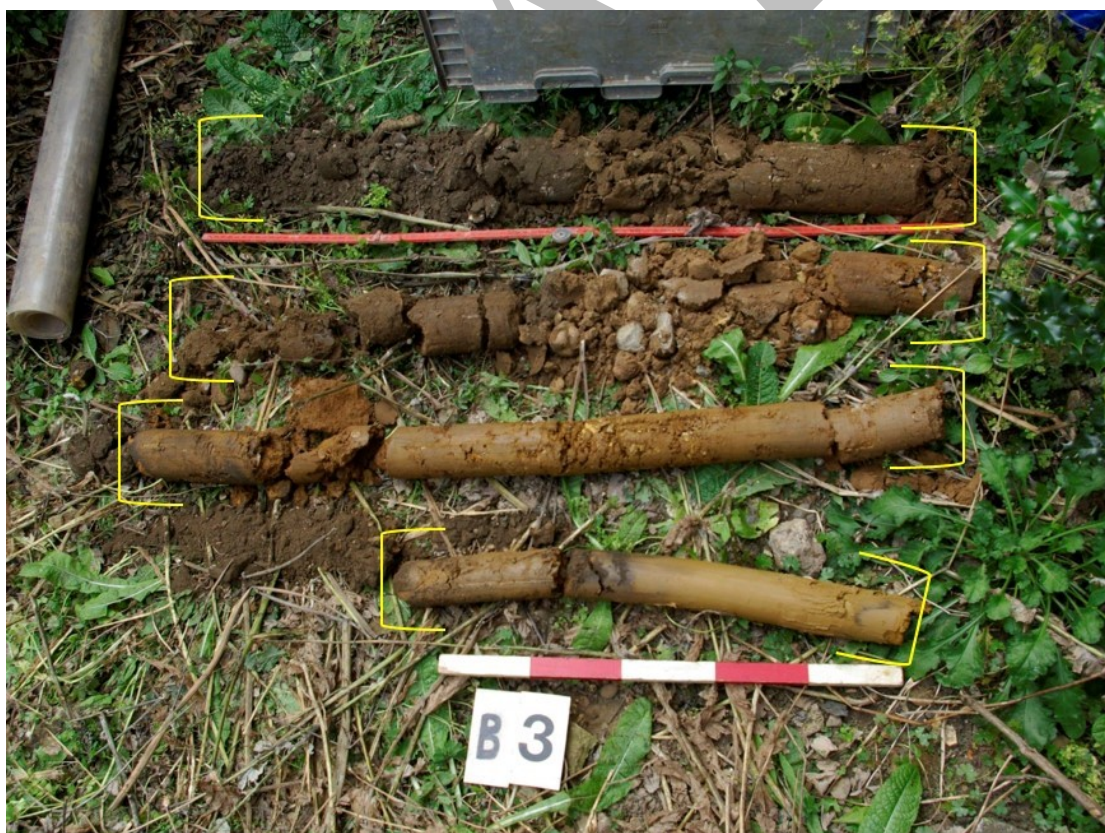
Figure 8 B3 borehole samples Samples highlighted by yellow brackets. 0.5m scale. Upper ends of samples to left
