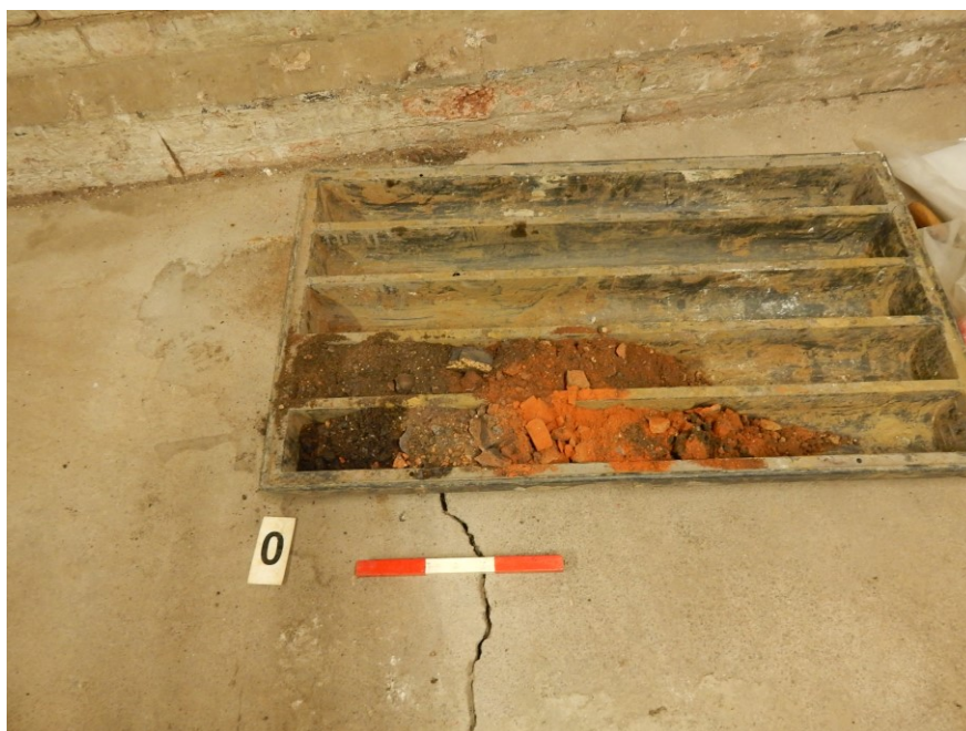
Figure 6 Core from Borehole 1 (0 top of the core)
