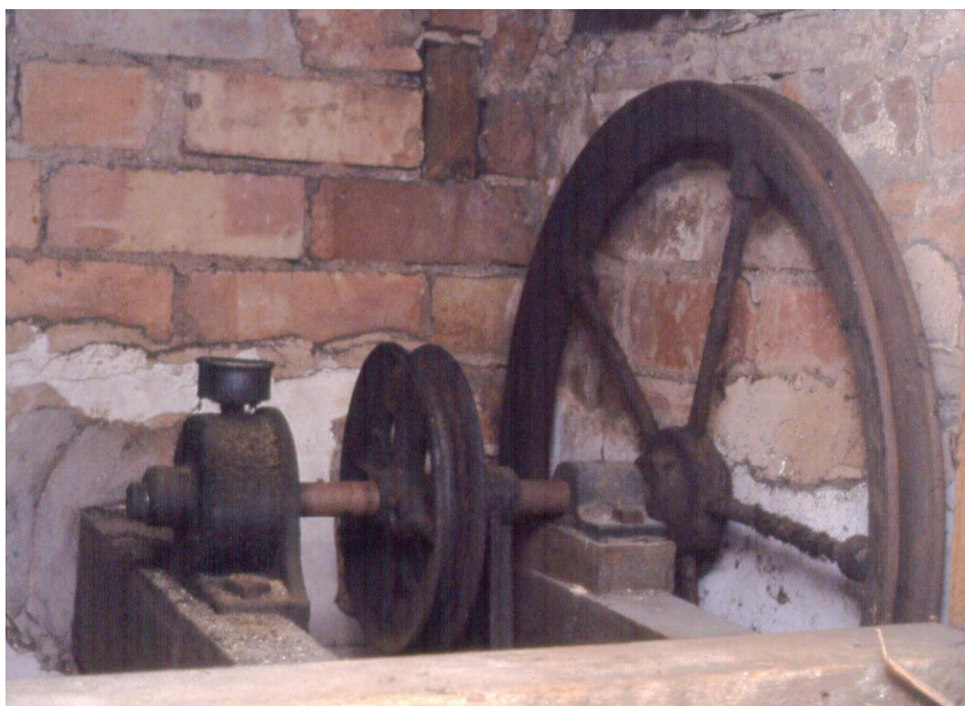
Plate 18 South cross wing, first floor: detail of dumb waiter mechanism
