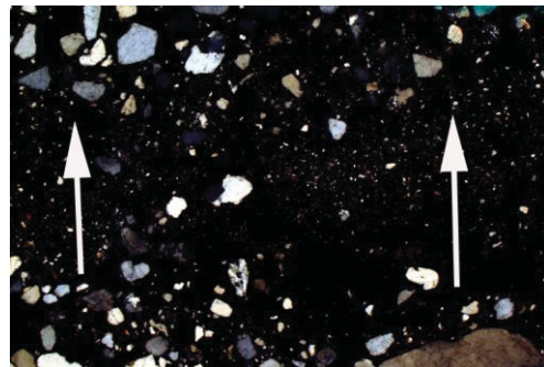
Figure 94: As Figure 93, under crossed polarised light (XPL); note inclusion of silt upwards (arrows).
