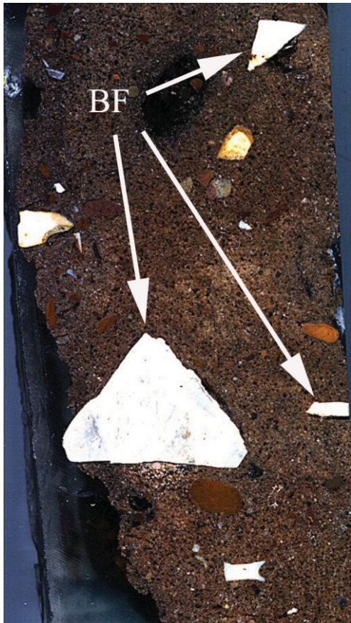
Figure 85: Enclosure Ib (M1, Context 170); macroscan of sliced impregnated block showing inclusion of coarse burned (calcined) angular flint (BF).
