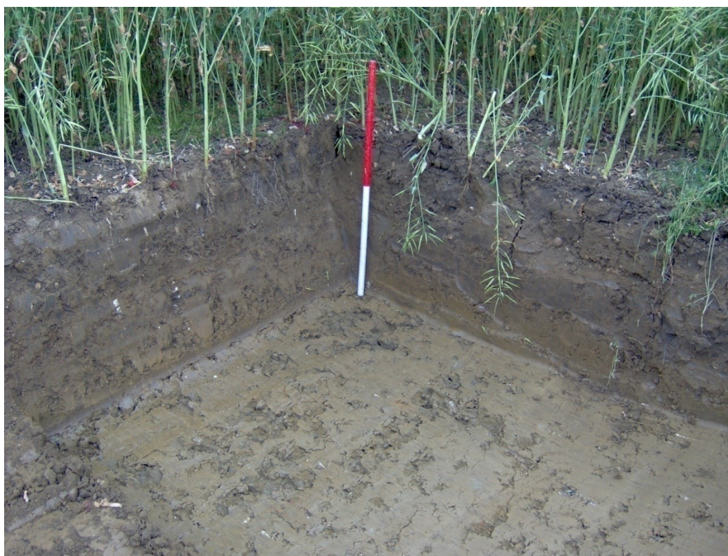
Figure 4: Northern corner of Turbine footing showing a typical section through the basic stratigraphic sequence of topsoil, subsoil and natural clay. Looking north.
