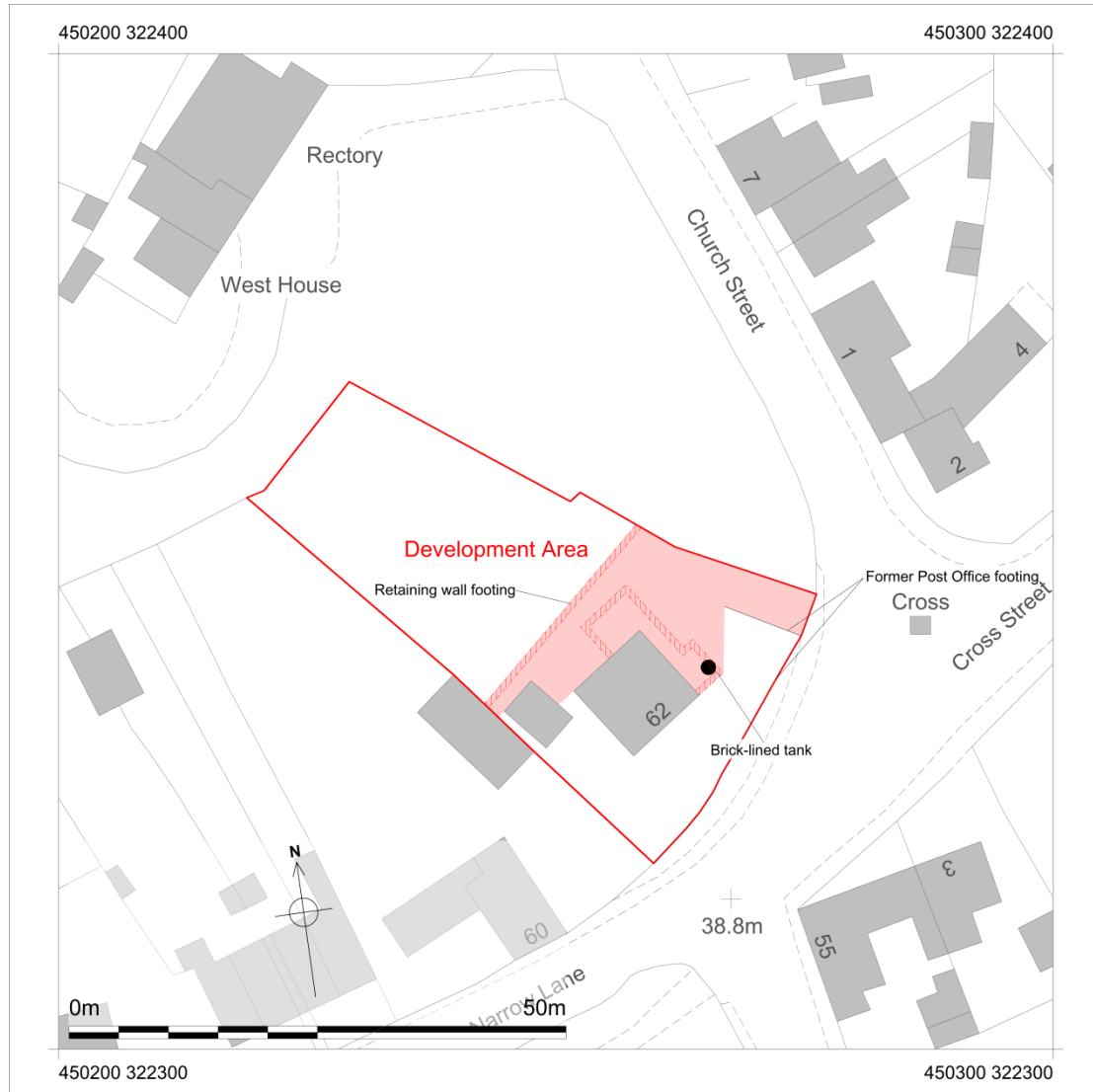
Figure 2: Development area showing area impacted by ground reduction and the location of the excavated foundation trenches
