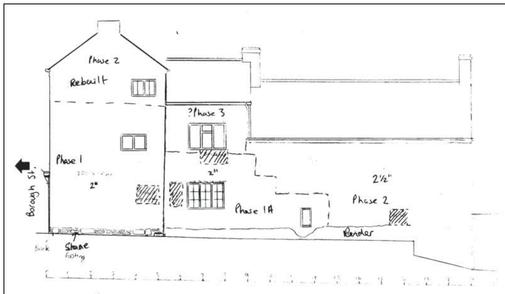
Figure 13: North elevation (adjacent to Co-op Supermarket) showing proposed building phases. The hatched areas denote bricked-in windows.
