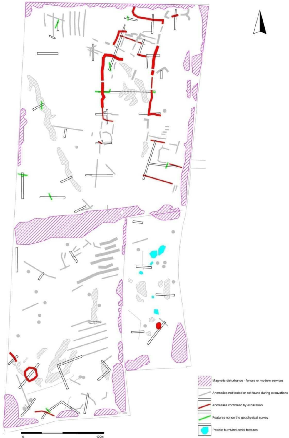
Figure 13 Trenches as excavated showing geophysical anomalies identified in excavation (red), those not tested or recorded (grey), features not identified on the survey (green) and other potential burnt/industrial features (cyan).
