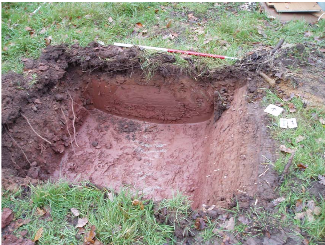
Figure 4 Test pit showing topsoil and Mercia Mudstone substratum viewed from the south
