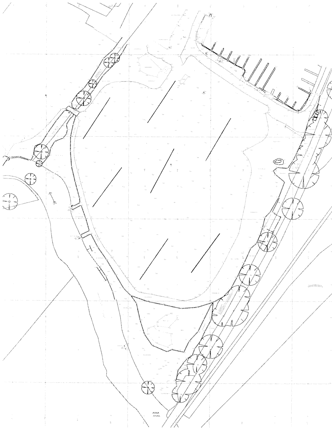
Fig 3 Topographical Survey with suggested trench locations
