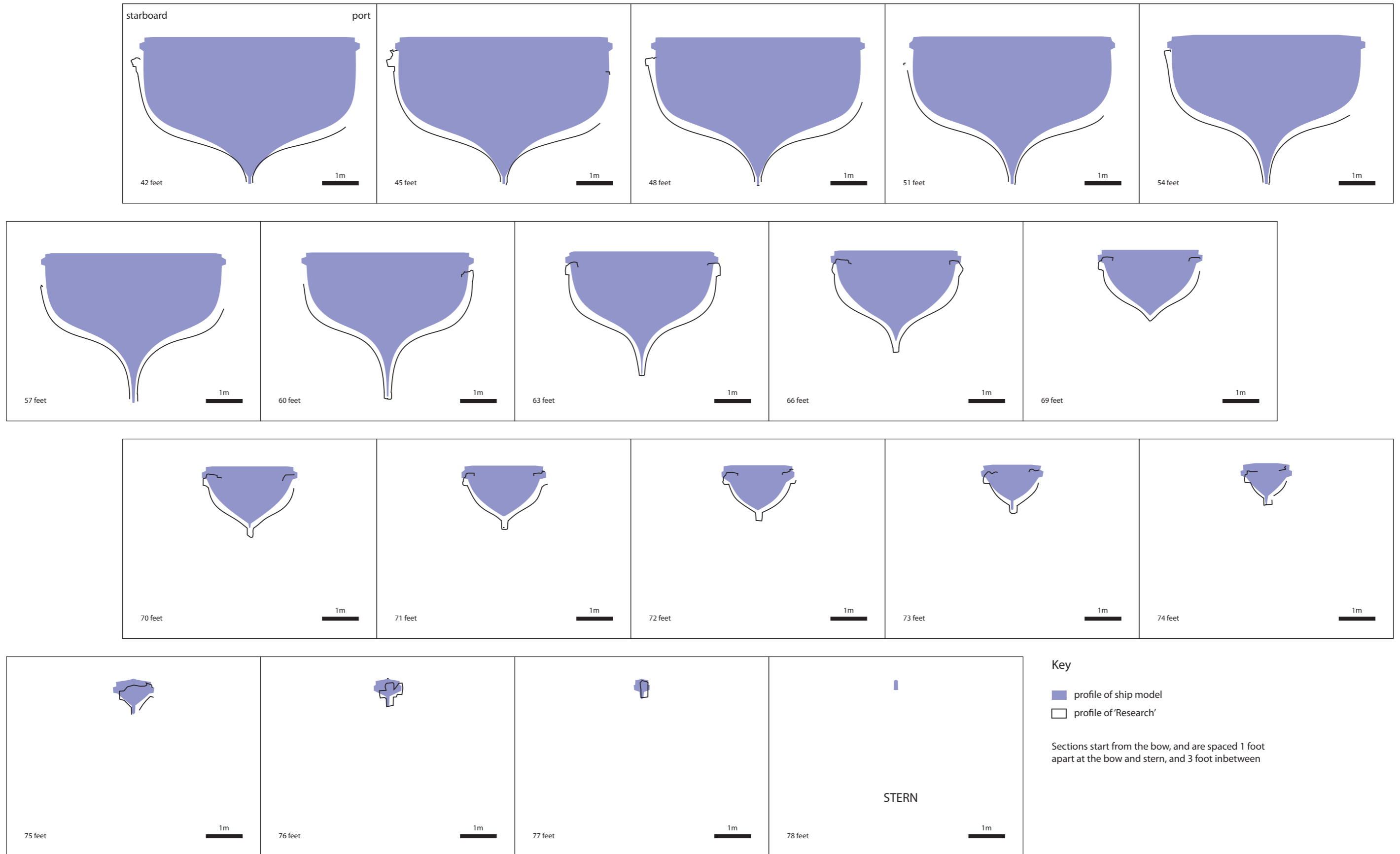
Illus A2.2 Comparative sections through the 'Research' and the shipbuilder's model
