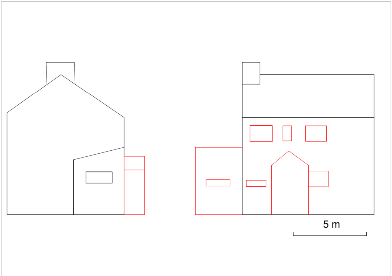
Figure 10. Sketches of the north (left) and west (right) facing elevations, red lines indicate 20 th century additions.
