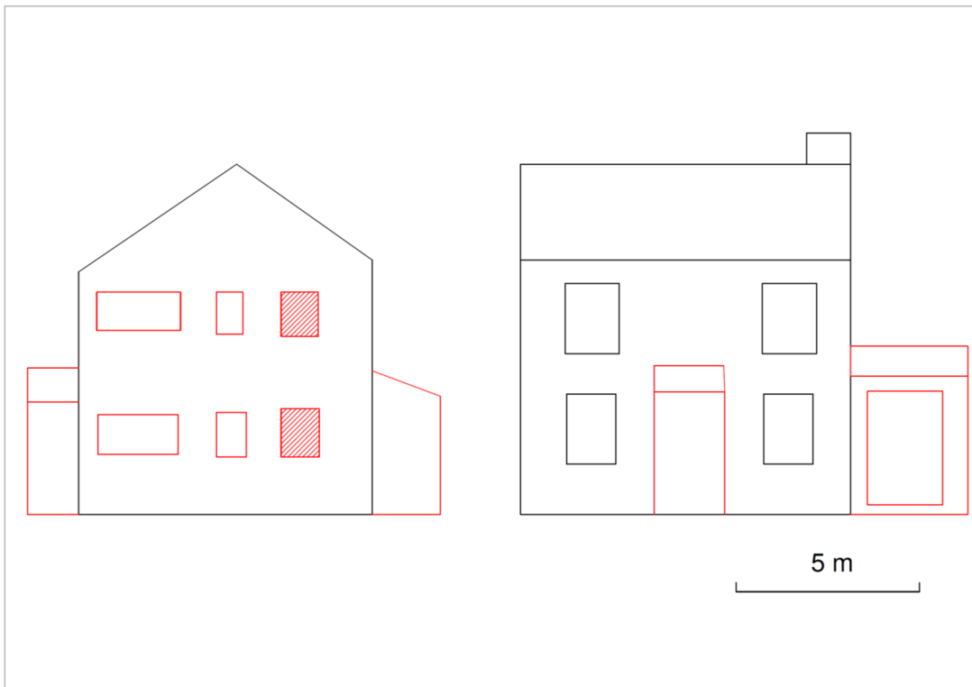
Figure 9. Sketches of the south (left) and east (right) facing elevations, red lines indicate 20 th century additions
