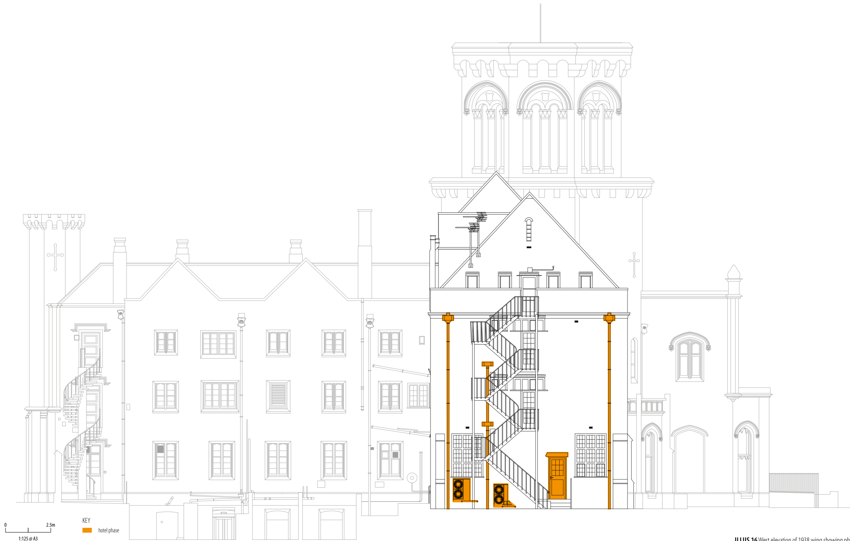
ILLUS 16 West elevation of 1938 wing showing phasing
