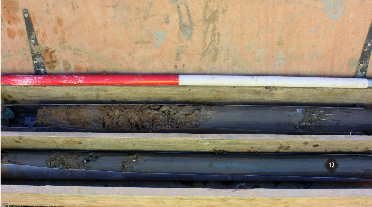
ILLUS 6 Cores from Borehole 106, 1–3m, BGL (1m BGL top left – 3m BGL bottom right). Sample 012 recovered from Group D - (10614) at 2.62–3.00m BGL
