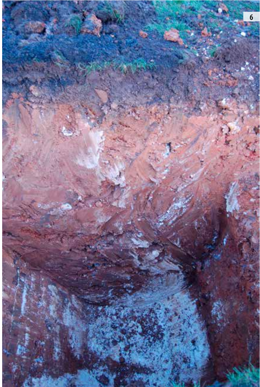
Test Pit 01: S facing section showing weathered Chalk surface and overlying Flinty Clay Plateau Drift
