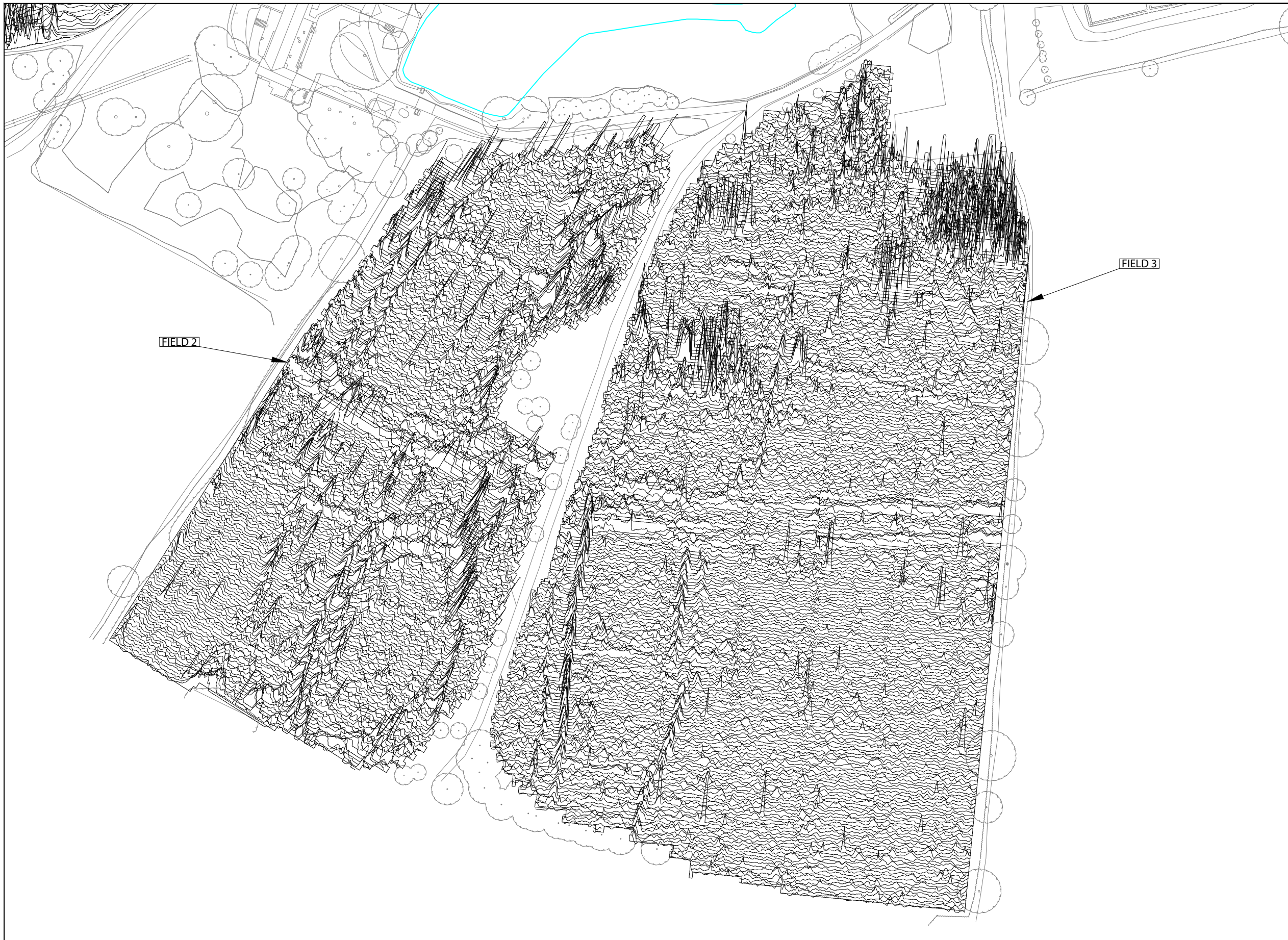
Illus 15 XY trace plot of magnetometer data; Field 2 and Field 3
