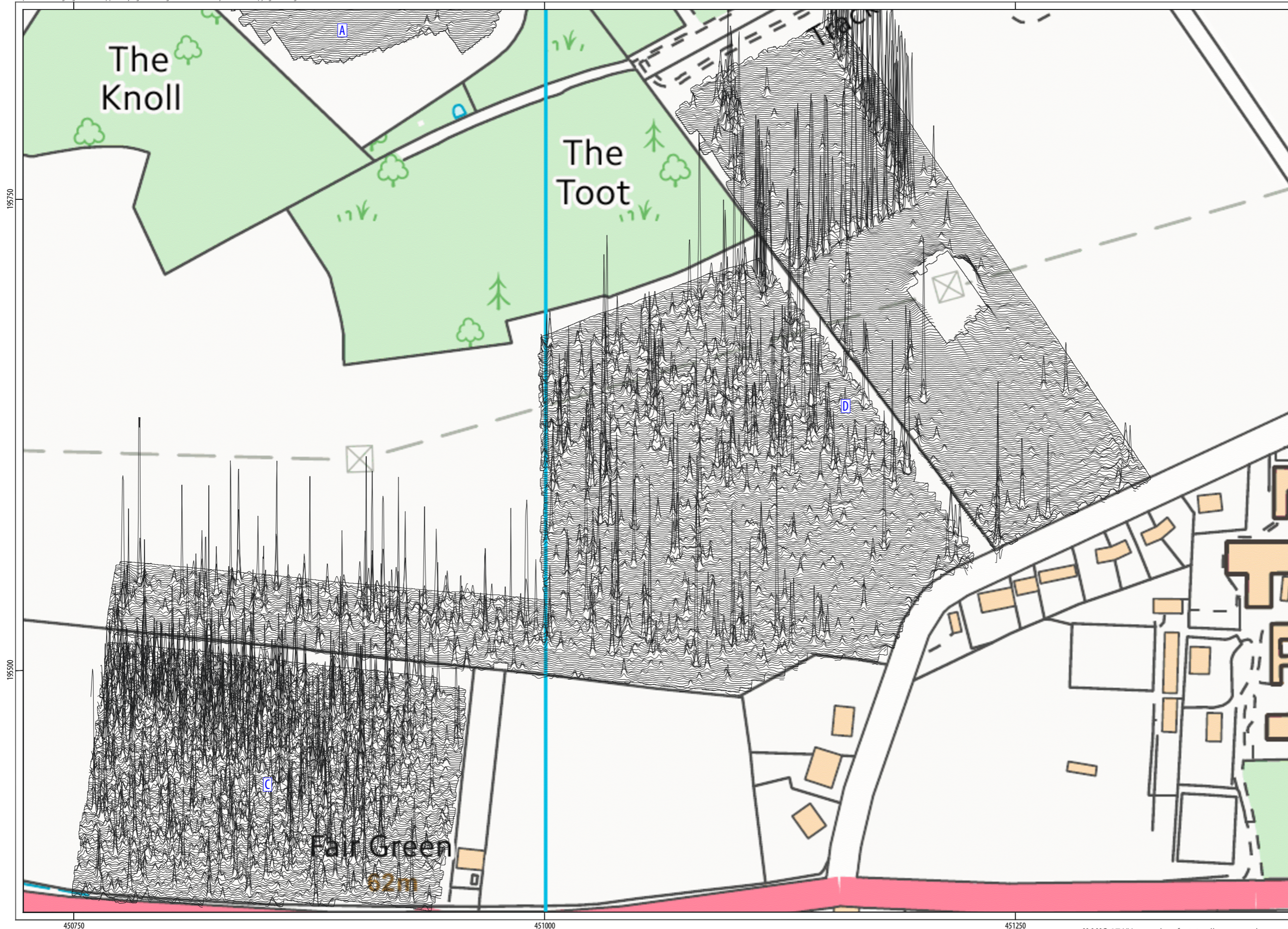
ILLUS 17 XY trace plot of minimally processed magnetometer data; Area C & Area D (1:2,000)
