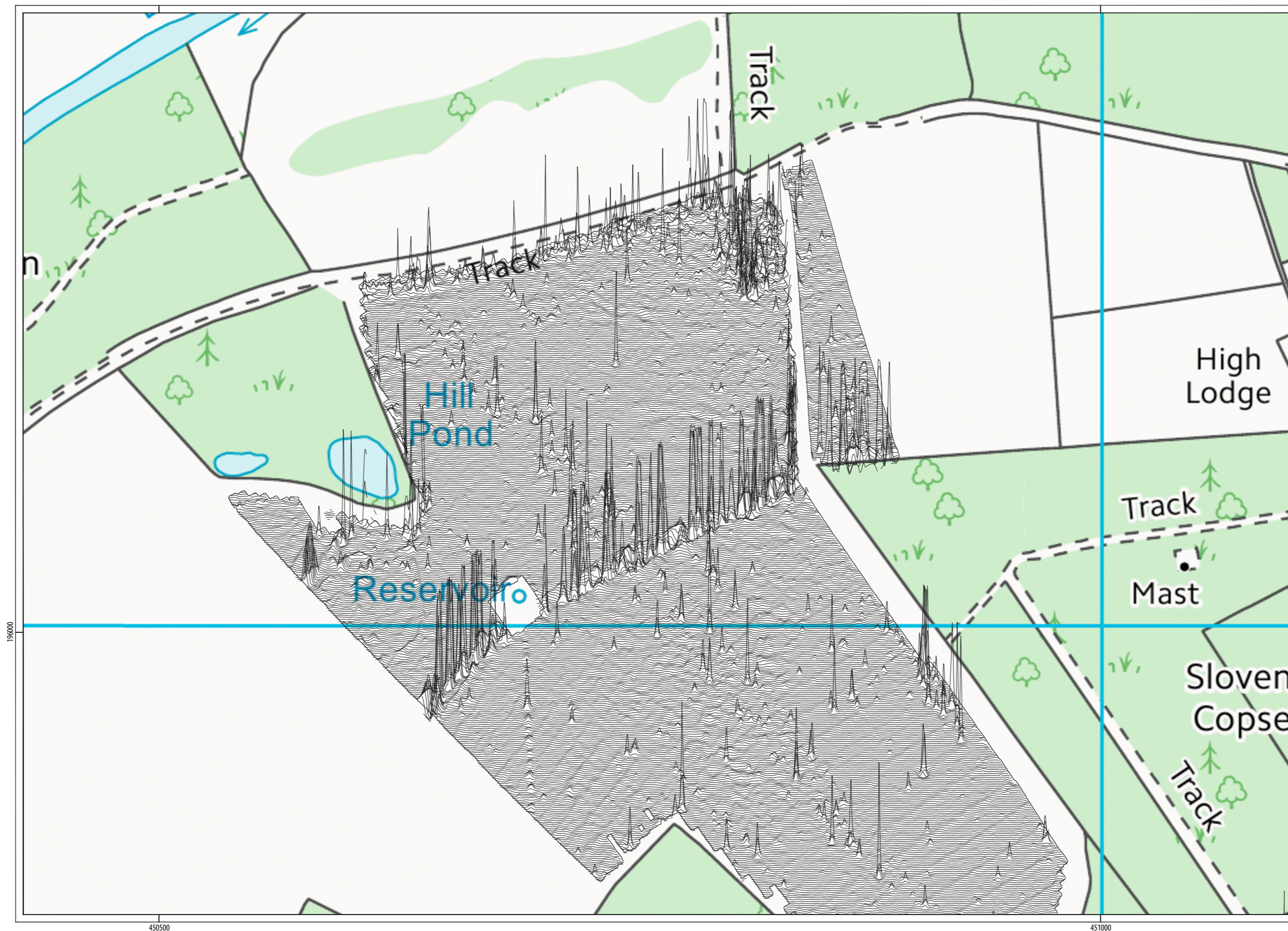
ILLUS 11 XY trace plot of minimally processed magnetometer data; Area A (1:2,000)
