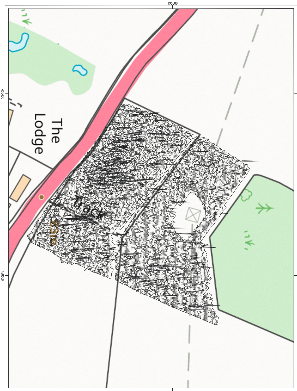
ILLUS 14 XY trace plot of minimally processed magnetometer data; Area B (1:2,000)
