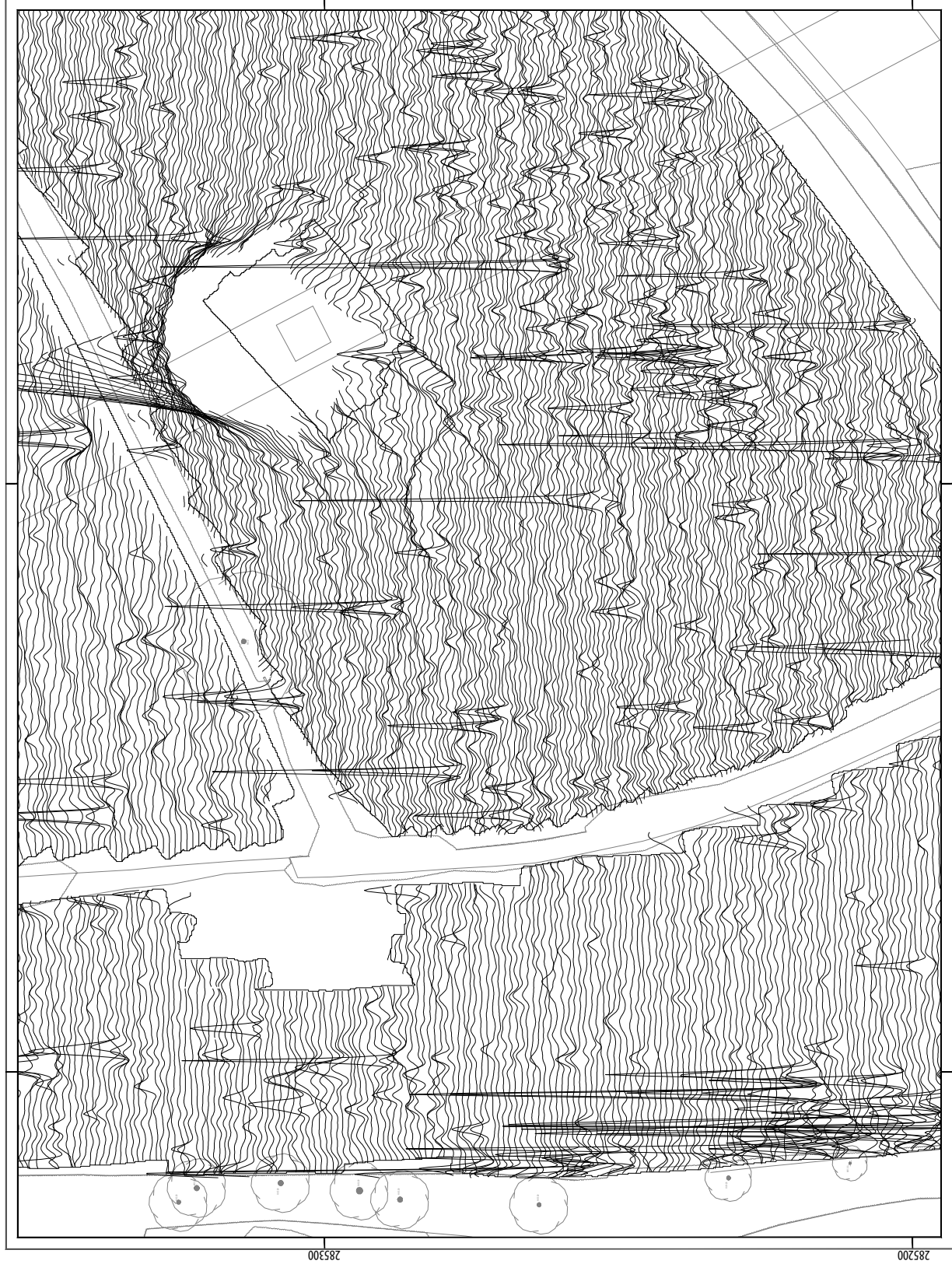
ILLUS 69 XY trace plot of minimally processed magnetometer data; AAA7
