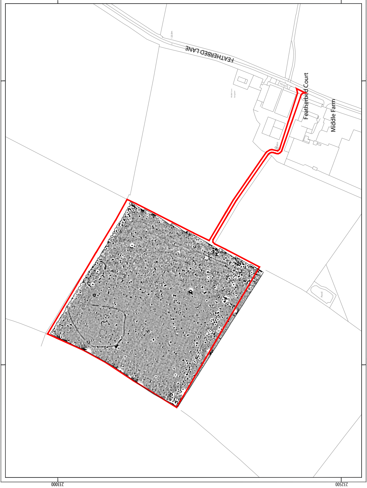
ILLUS 4 Processed greyscale magnetometer data (1:4000)
