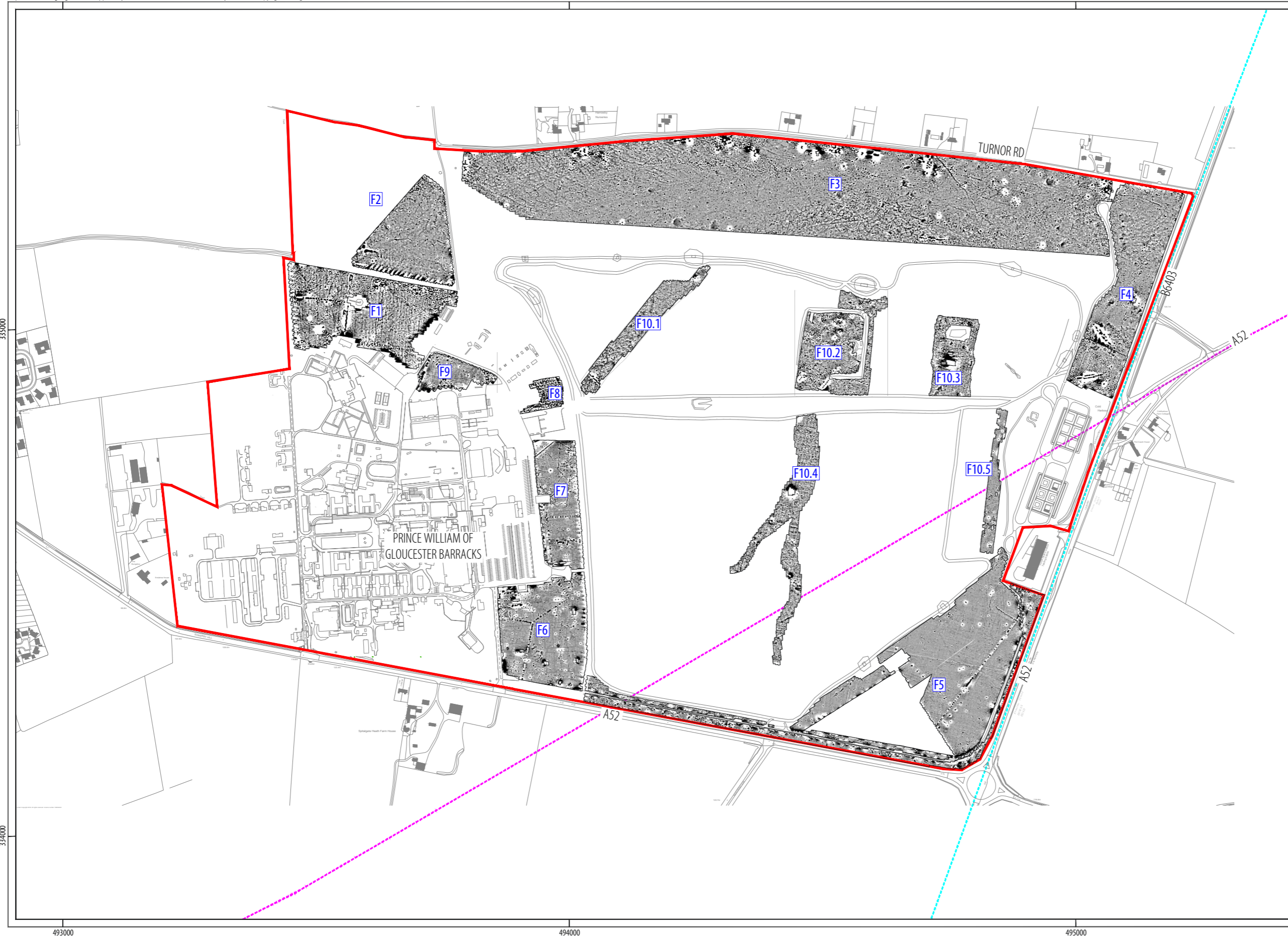
ILLUS 8 Processed greyscale magnetometer data (1:7,500)
