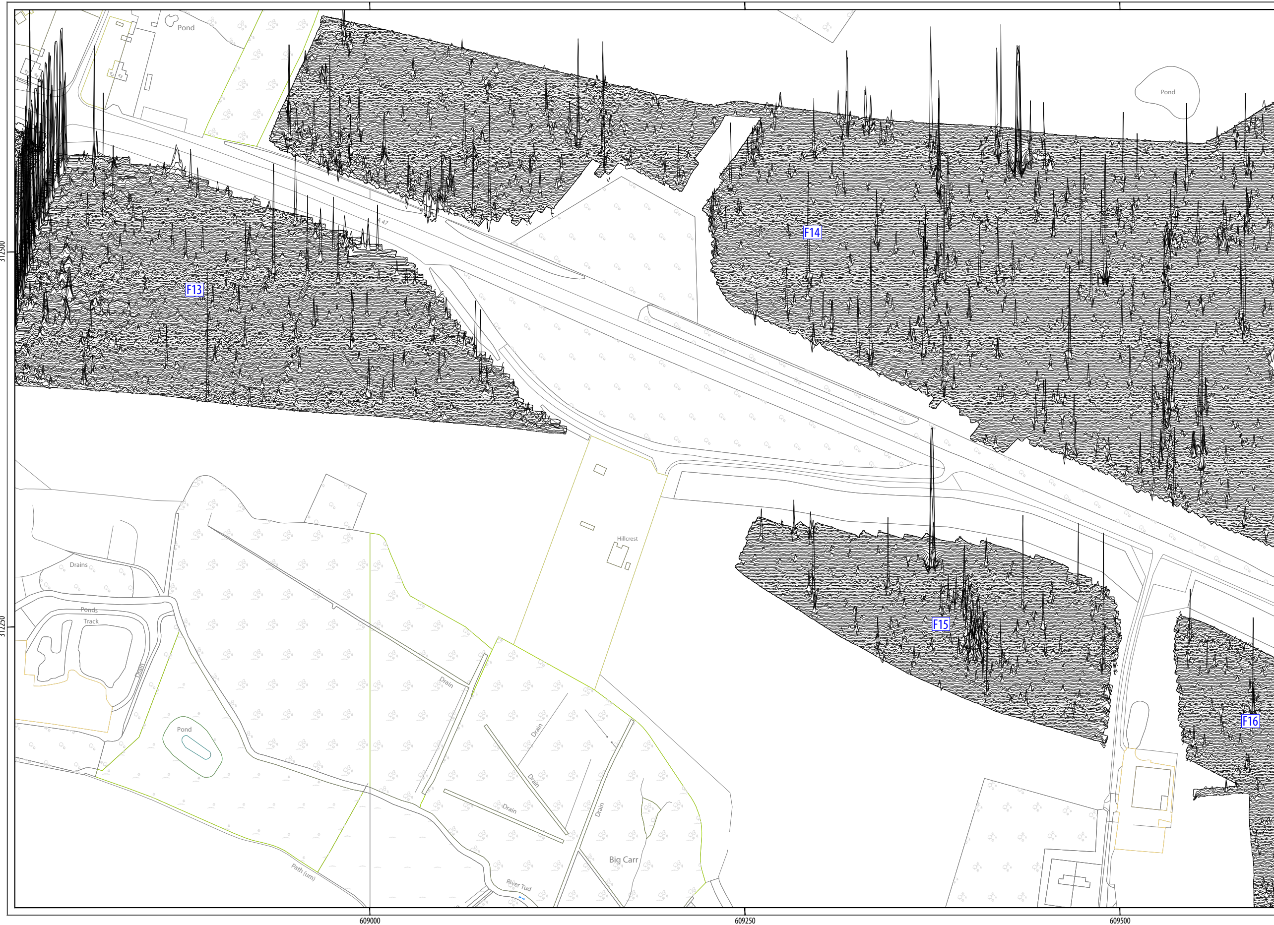
ILLUS 27 XY trace plot of minimally processed magnetometer data; Sector 5
