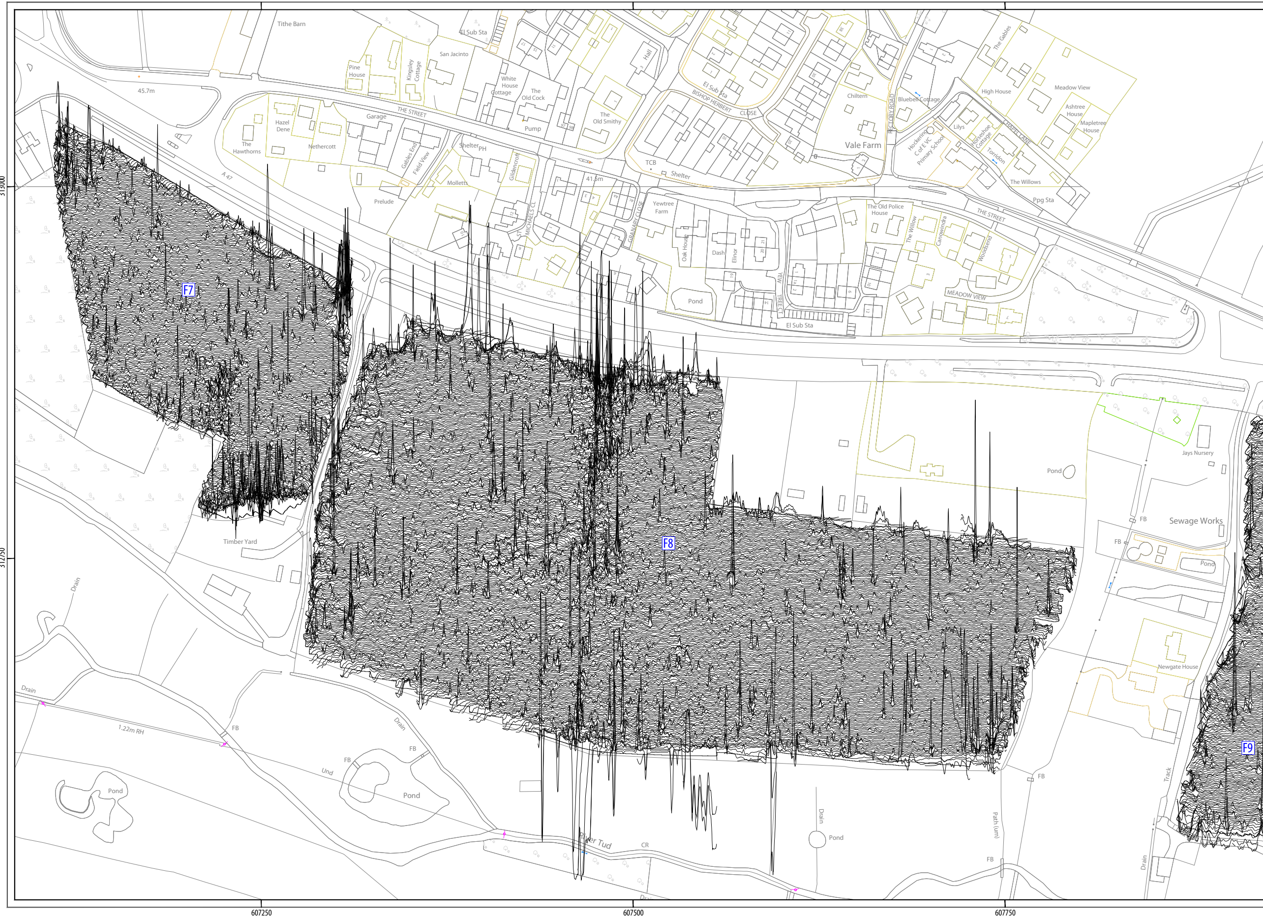
ILLUS 21 XY trace plot of minimally processed magnetometer data; Sector 3
