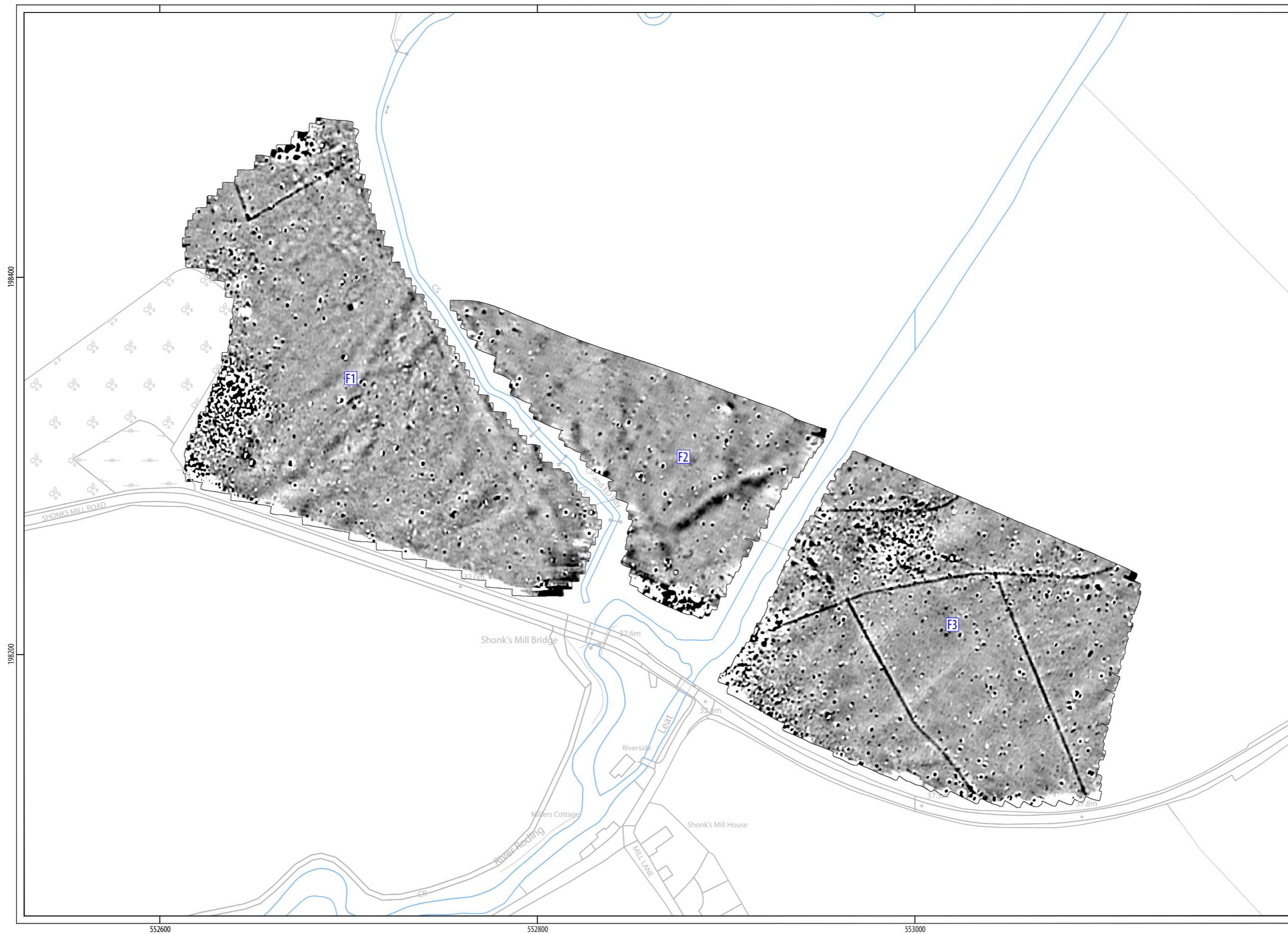
ILLUS 6 Processed greyscale magnetometer data (1:2,000)
