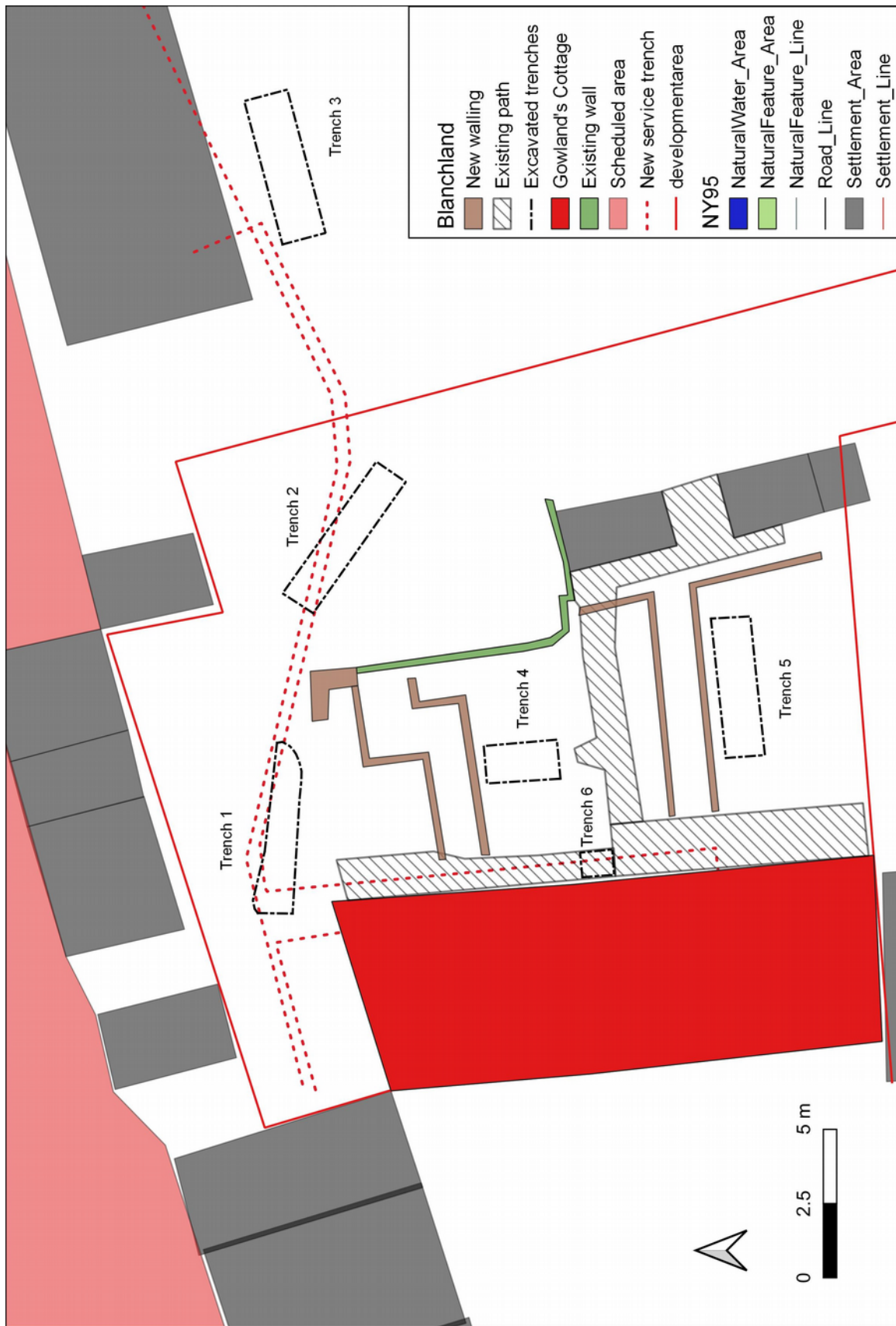
Figure 4: The site area showing the proposed new structures and trial trench location
