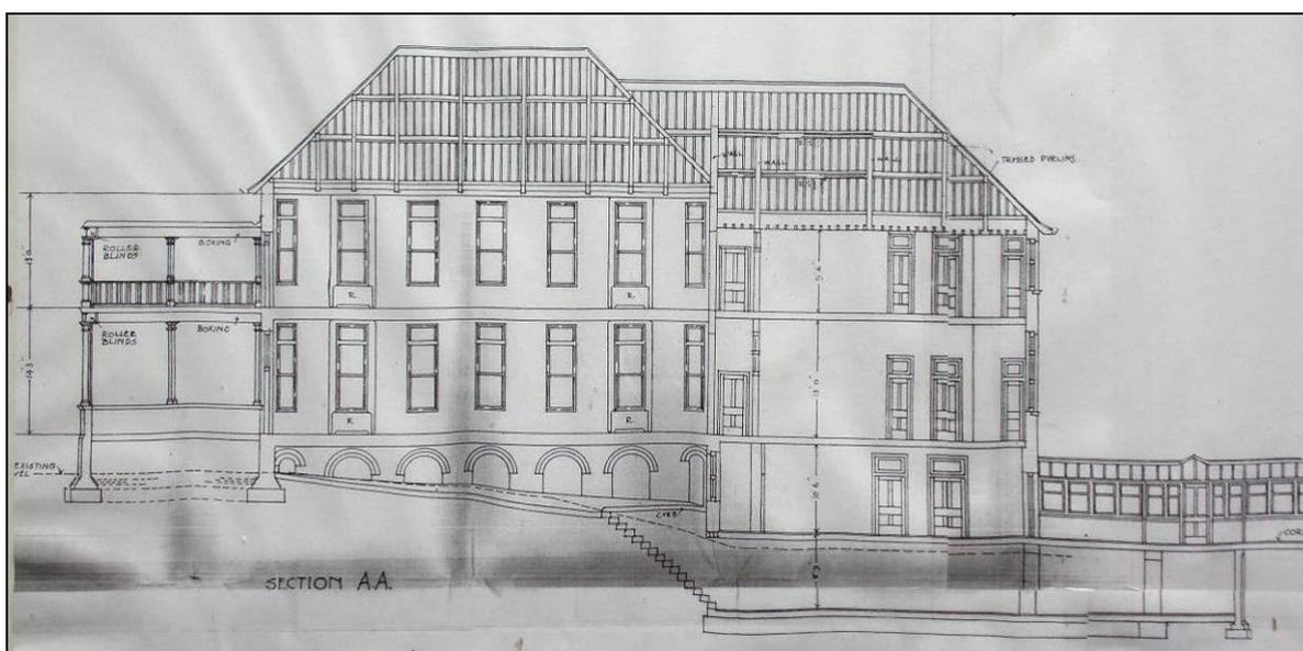
Figure 7: Copy of original architectural drawing of Building 41 showing a longitudinal section.
