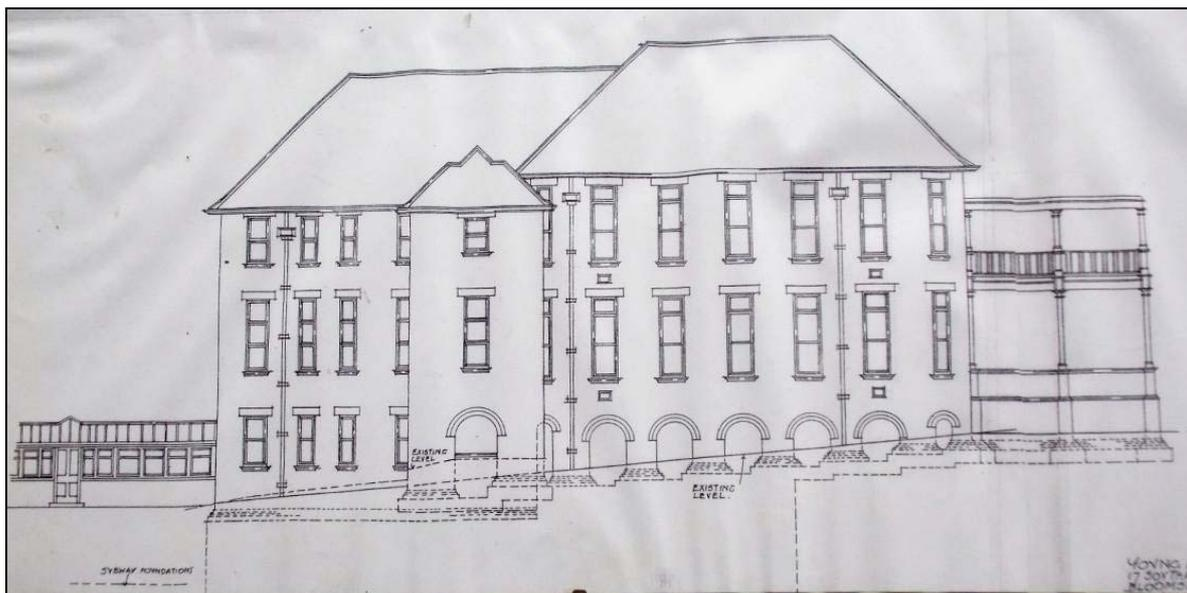
Figure 6: Copy of original architectural drawing of Building 41 showing the west elevation.
