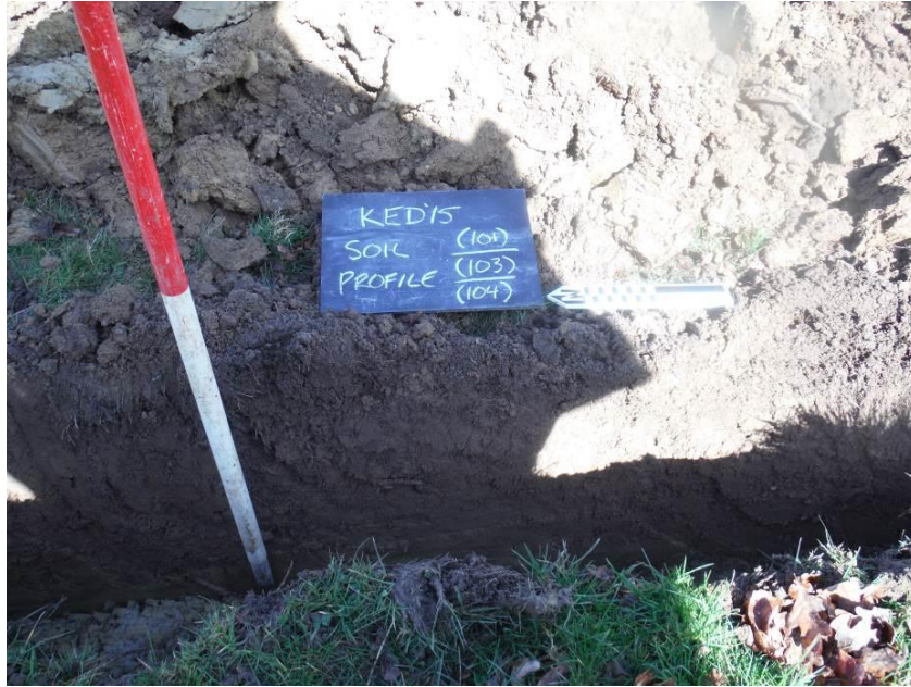
Figure 4. Soil profile of topsoil (101), mid-brown subsoil (103) and mottled grey and yellow clay (104). Scale 1m.
