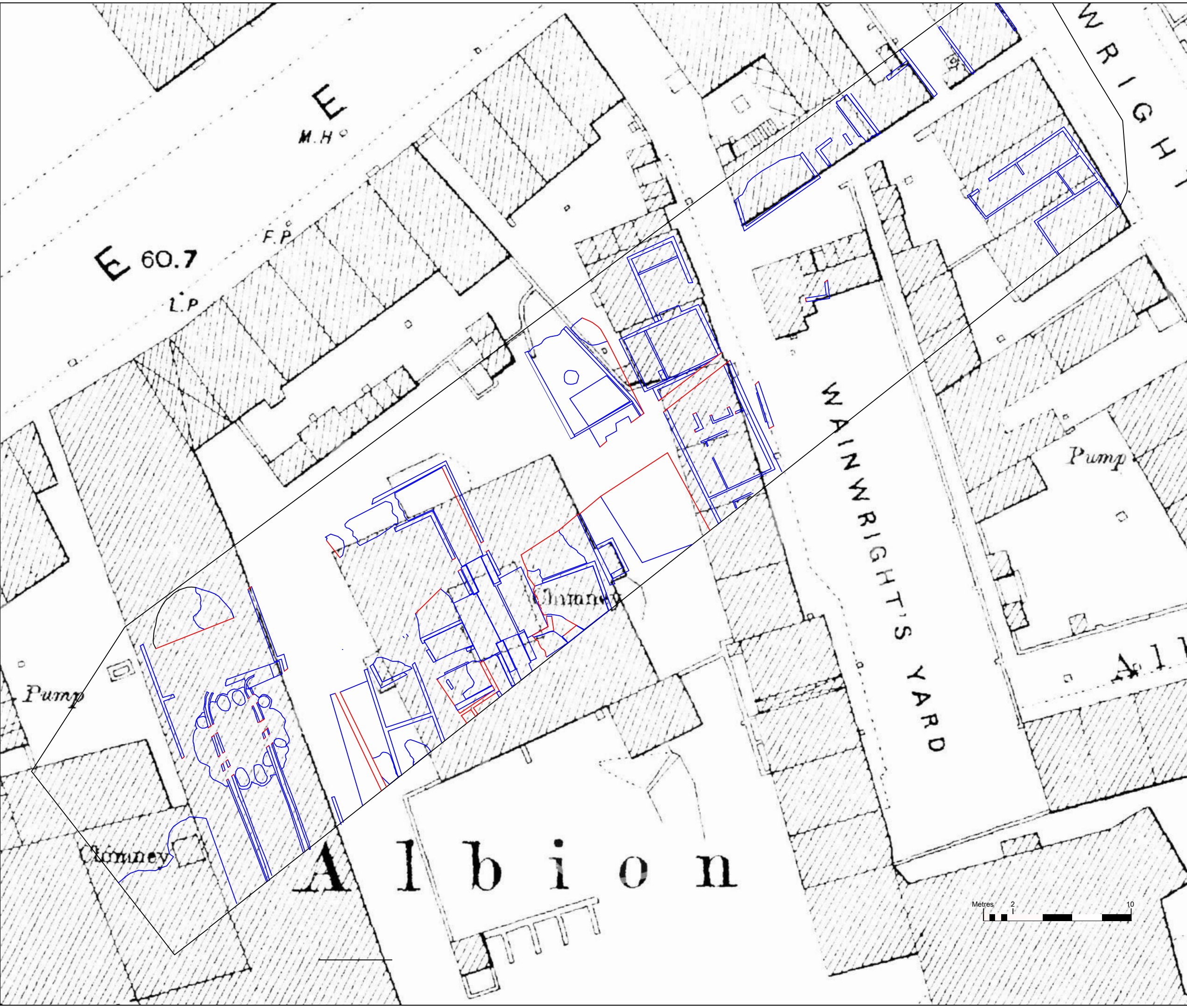
Figure 92- Plan of Excavated Features with 1890's OS Map Overlay Scale: 1:250 @ A3 Drawn: RL
