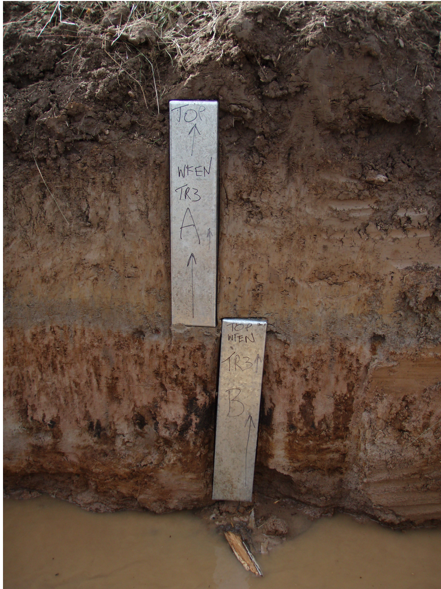
Figure 9. Two monolith tins in position, prior to extraction
