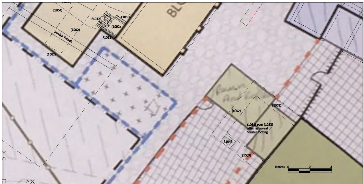
Figure 5. Plan showing excavated area for new Block A outbuilding. Note alignment of the service trench (top left) with the manhole (F1048). Scale: as shown.
