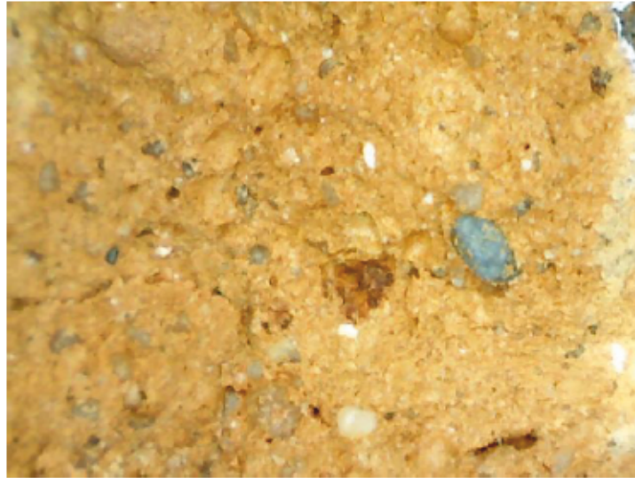
Figure 25 - Fresh break of CBM fragment at 10x magnification.
