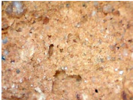
6mm wide cross-section for a fresh break of TZ11
