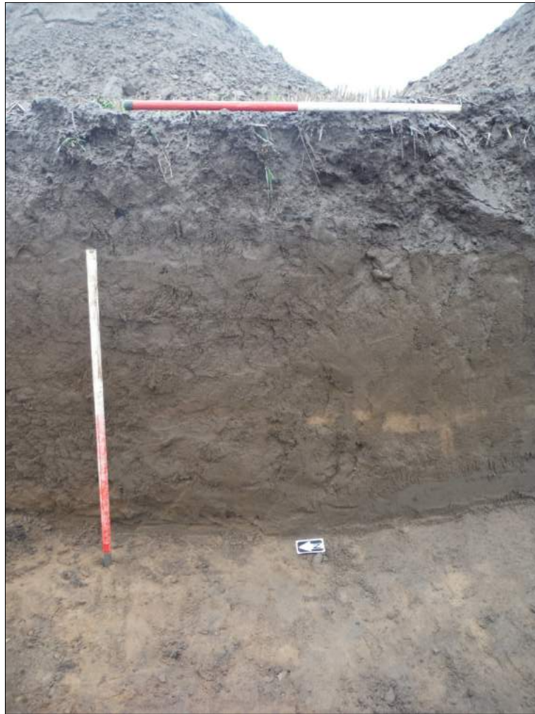
Figure 40. West facing representative section of Trench 79 showing paleochannel [7906] showing alluvial layers (790; 7905) (scale = 2x2m in 0.5m graduations).
