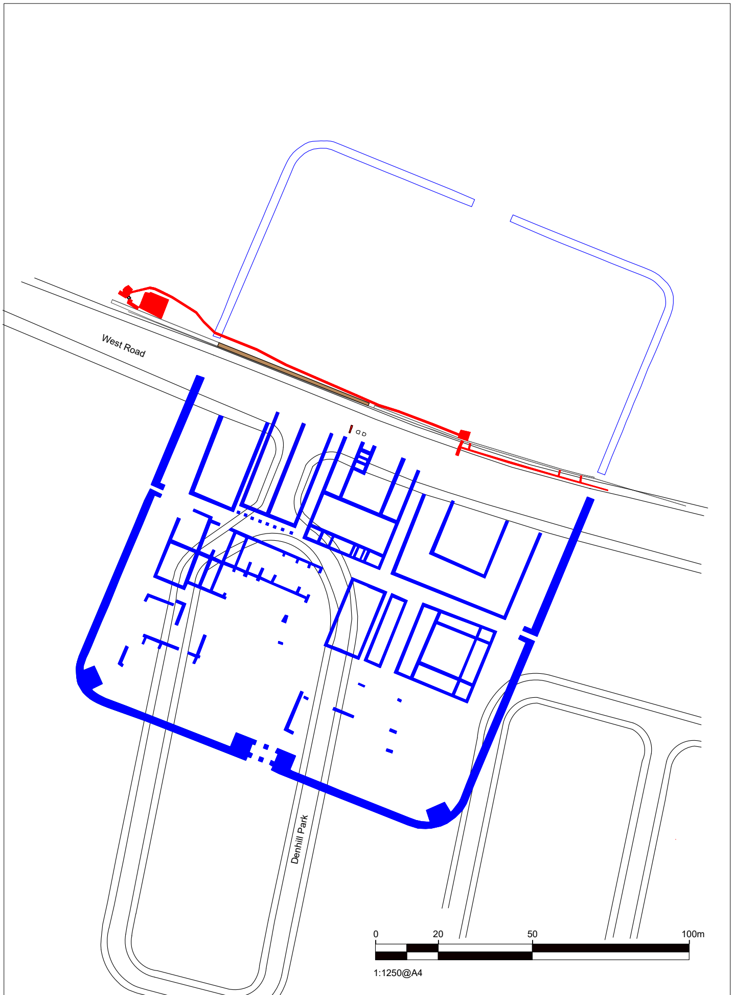
Figure 21. Plan of Condercum Fort overlain by the current road layout, and service trench locations
