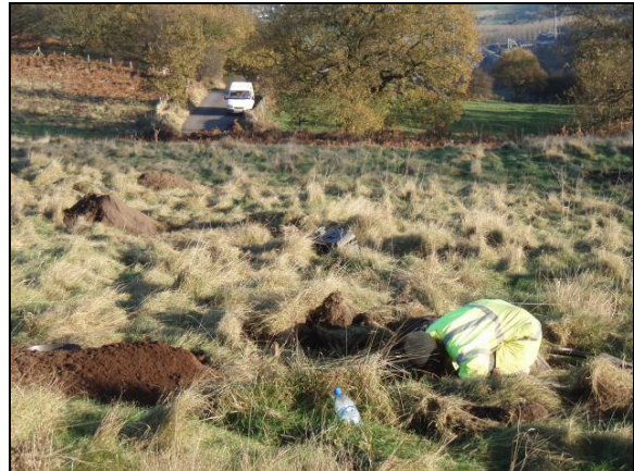
Excavation of a test pit at Birchover Quarry.
