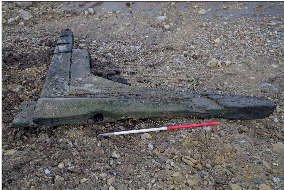
Plate 28: Sternpost, keelson and deadwood knee showing hole for propellor shaft from Hulk 1
