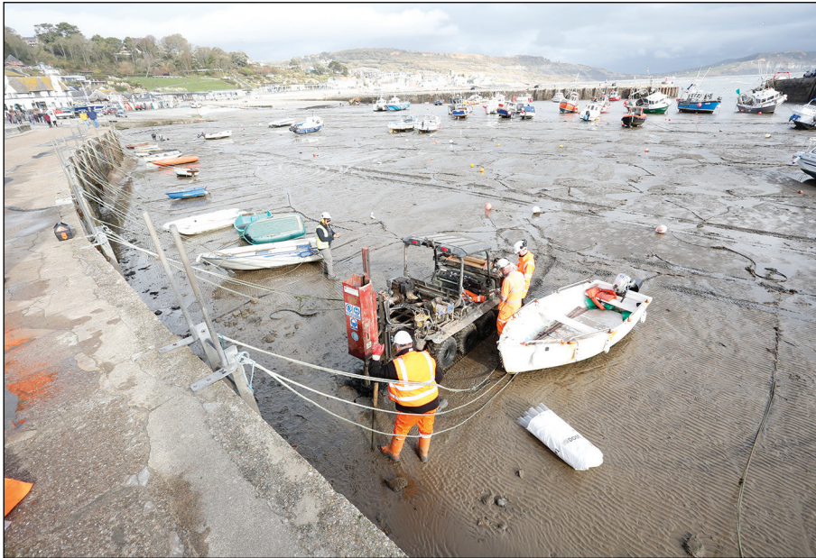
Plate 17: Window sample 105, percussive technique.
