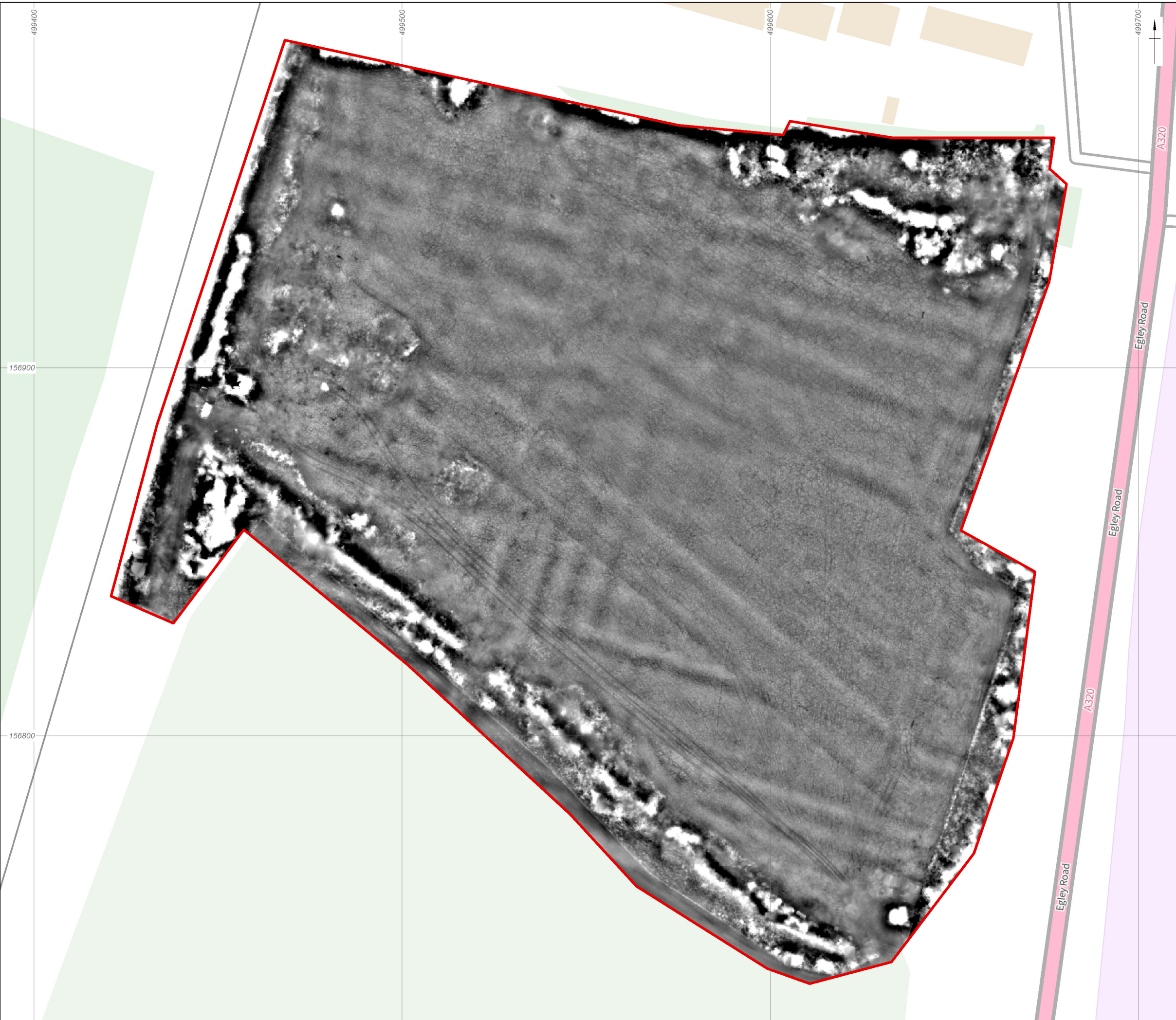
Figure 3: Local Relief model created from a 20cm Digital Terrain Model
