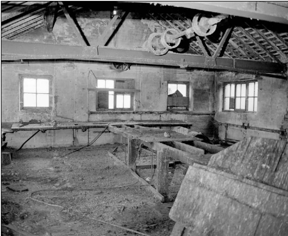
Plate 393: General view of S5, north range – note workbenches and overhead line shafting (film 45.4)
