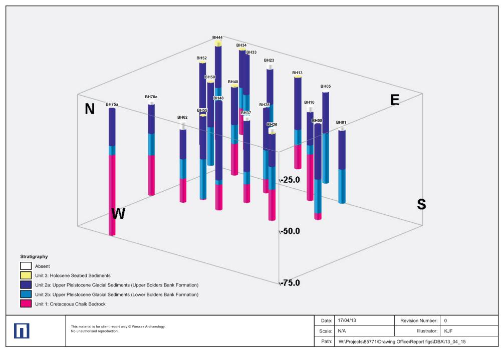
Rockworks Borehole model Figure 2
