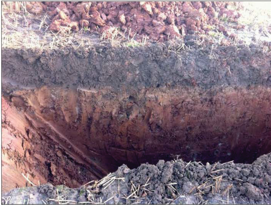
Plate 1: Test Pit 11, representative section showing soil leaching
