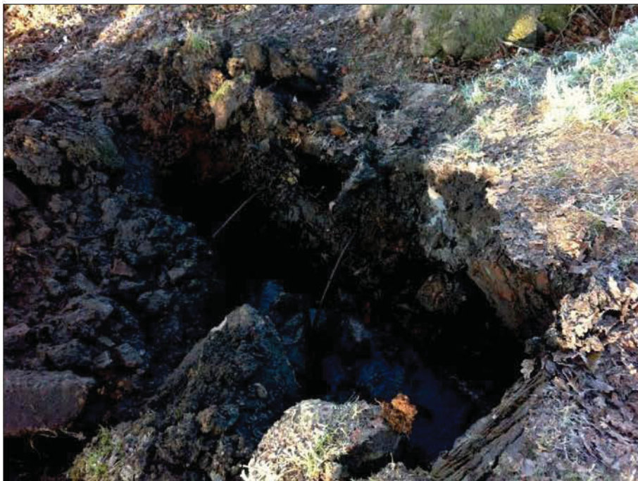
Plate 2: Test Pit 101, showing made ground
